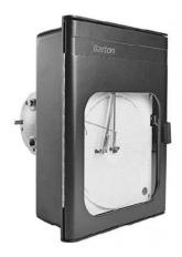
Barton Two Pen Pressure Temperature Recorder, Model 242E, Pressure Range: 0-600 Psi, Mechanical Chart Drive: 24 HRs/7 Days
