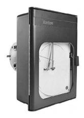
Barton Two Pen Pressure Temperature Recorder, Model 242E, Pressure Range: 0-3000 Psi, Mechanical Chart Drive: 2 HR/ 8 HR
