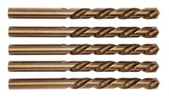
Due to the inclusion of 5% cobalt to their alloys, the Kennedy line of heavy duty straight shank jobber drills with HSS-Co delivers dependable and long-lasting cutting performance at high temperatures and speeds. They can drill steels with tensile strengths of up to 1,400 N/mm2, very hard bronze, stainless steels, as well as steels that are heat- and acid-resistant thanks to their toughness and heat resistance.
