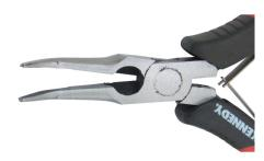
Dissipative handles safely discharge any electrostatic energy, reducing possibility of damage to sensitive items. The dual material grip handle design allows the user to apply the greatest force with the minimum amount of effort. These are manufactured with a polypropylene core for strength and durability with a soft thermoplastic outer for non-slip comfort grip.
