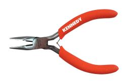
Manufactured from heat-treated stainless steel. Hardness: pliers: 42 - 45HRC; nippers: 45 - 48HRC. Used for delicate, fine and accurate work in a continuous production environment. With cushioned foam safe-grip handles for user comfort and control. Spring-loaded return for quick repetitive opening and operator comfort. Cushioned foam safe-grip handles for user comfort and control.
