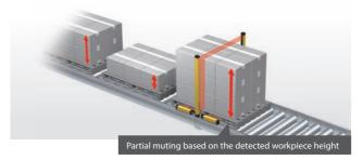
\* Partial muting: A function that allows specified beams (e.g., beams blocked by a workpiece) to be disabled, keeping others active, even during muting.
