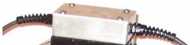
When either activation system is activated, there is a ½ Watt control signal sent to the Module (semiconductors) sealed in the Output Module. The Output Module connected to a receptacle plug on the reverse side of the Control Panel, and supplies the necessary power to the encapsulated Coil.
